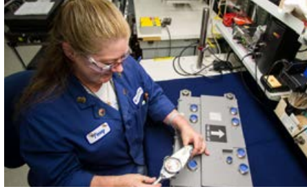
A UTC Aerospace Systems technician in Windsor Locks, Conn., performs final assembly checks on a PW1500G Full Authority Digital Engine Controller.
