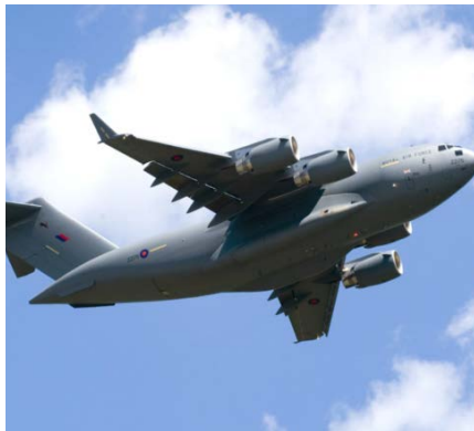
The Royal Air Force flies eight C-17 Globemaster aircraft, each powered by four Pratt & Whitney F117 engines. The large military transport aircraft is designed to carry equipment, supplies and troops to small airfields in harsh terrain anywhere in the world, day or night.
