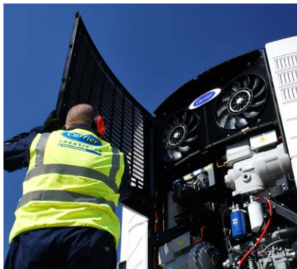
In 2016, U.K. food retailer Sainsbury's became the first customer to take delivery of Carrier Transicold's prototype natural refrigerant trailer unit. The next-generation system uses low global warming potential carbon dioxide refrigerant, a safe and non-ozone depleting gas that sets the standard for refrigerants and supports advances toward a smart, sustainable cold chain.
